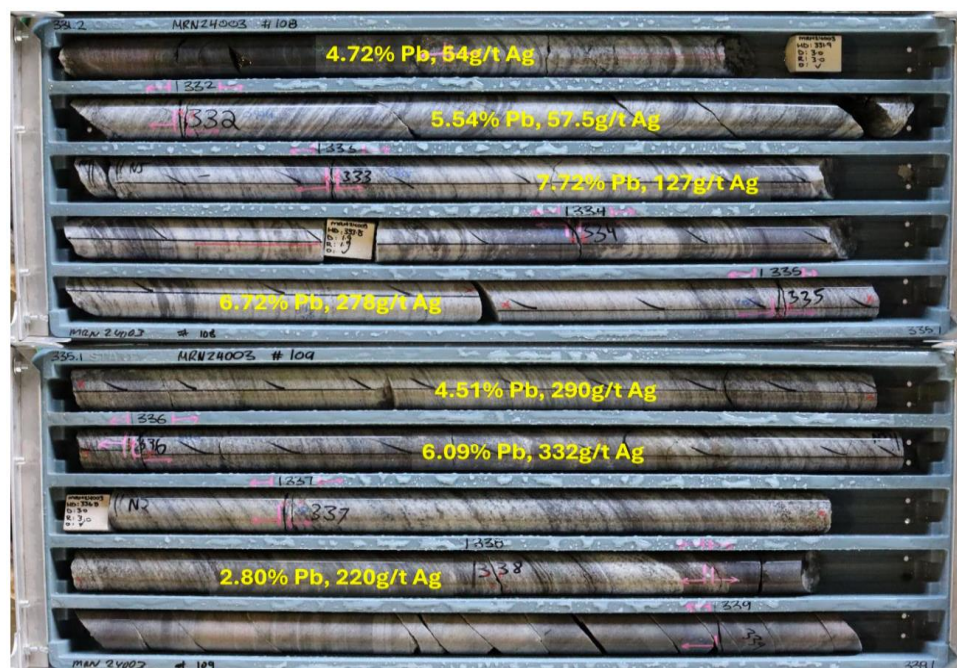
Figure 9: Core with marked grades from soft carbonate lead-silver ore type
